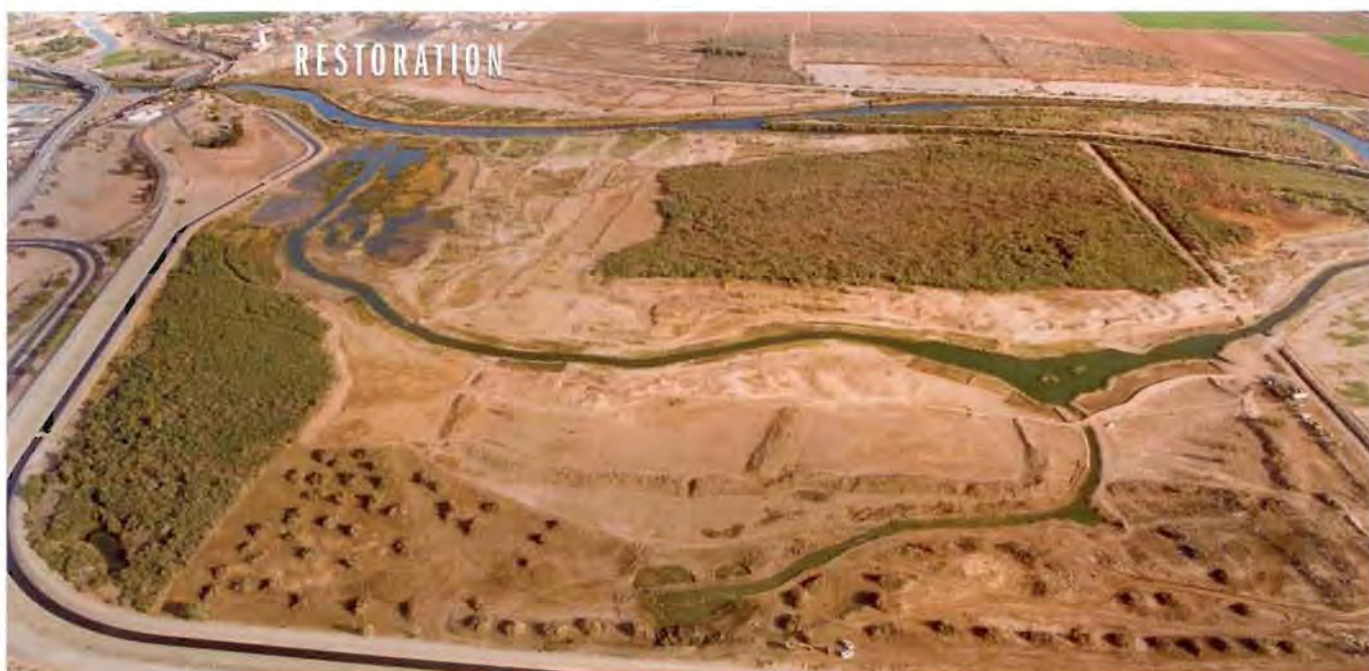
The YEW south channel project during construction shows piles of tamarisk ( above , in the foreground, and below ) that await burning. An "after" photo, bottom , shows the same area flooded with pumped groundwater and infrequent high river flows.
