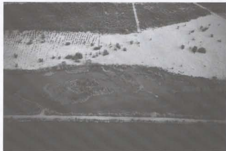
'Ahakhav backwater and revegetation site three months after planting. Note grid of transplants in upper left of cleared area. Isolated from the river, and no longer scoured by floods, backwaters such as this one act like desilting ponds, gradually filling with sediment that must be removed to allow for restoration of the backwater ecosystem.
